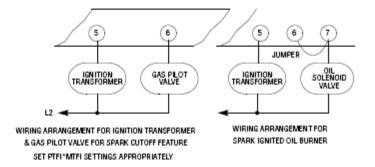
Caution: All safety limit switches should be approved as limit controls and should be wired directly in the circuit of the Flame Safeguard control. The use of electronic switches to close interlock circuits may cause erratic operation.
