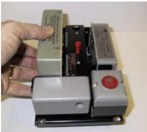
Fig. 47 D Series chassis, module retainer removed, showing insertion of amplifier module.
