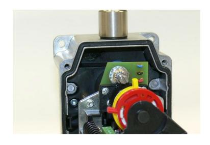
Factory Default Direction "Anti Clockwise" (CCW) Position of Limiters
