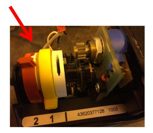
Connect new servo to coupling and check travel
