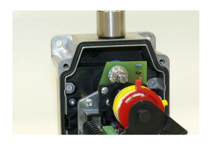
Alternate Direction "Clockwise" (CW) Position of Limiters
