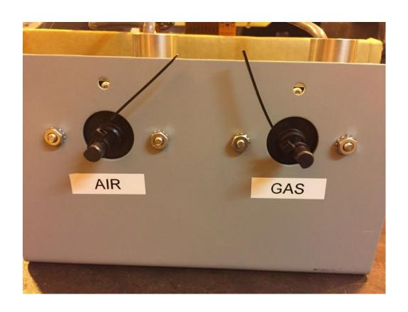
Note the position of the flat on the gas servo. It drives CW to open.
