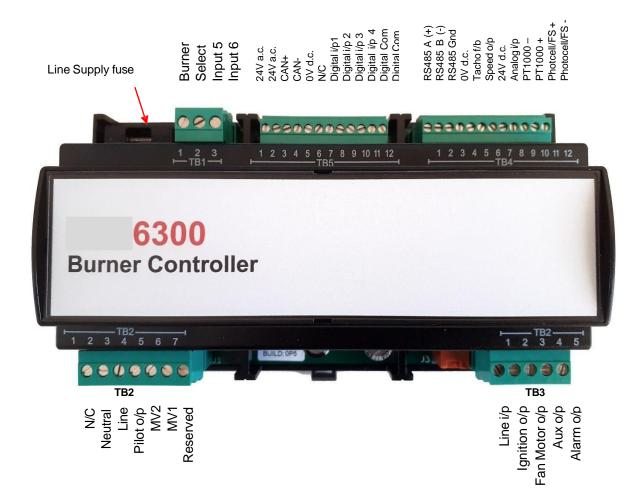
Each terminal set has a removable block to make wiring a little easier. The terminal blocks must be pushed fully home to ensure reliable operation.
