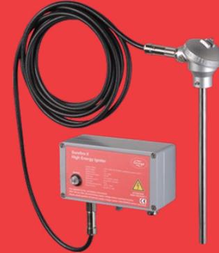
The SureFire II High-Energy Ignition System is used for direct spark ignition of most gas or liquid fuels used in oil or gas igniters or main burners. The High-Energy Ignition System is available in various versions. To ensure optimal operation, the first part of the ignition tip should always be in an ignitable fuel-air mixture, during all modes of operation.
