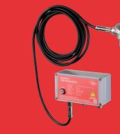
The SureFire II High-Energy Ignition System is used for direct spark ignition of most gas or liquid fuels used in oil or gas pilots or main burners. The High-Energy Ignition System is available in various versions. To ensure optimal operation, the first part of the ignition tip should always be in an ignitable fuel-air mixture, during all modes of operation.
