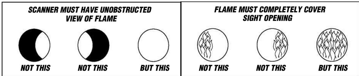
5. Smoke or unburned combustion gases absorb ultraviolet energy. On installations with negative pressure combustion chambers, a small hole drilled in the UV1AL sight pipe keeps the pipe clean and free from smoke. For positive pressure furnaces, provide clean air to pressurize the sight pipe, if necessary.
