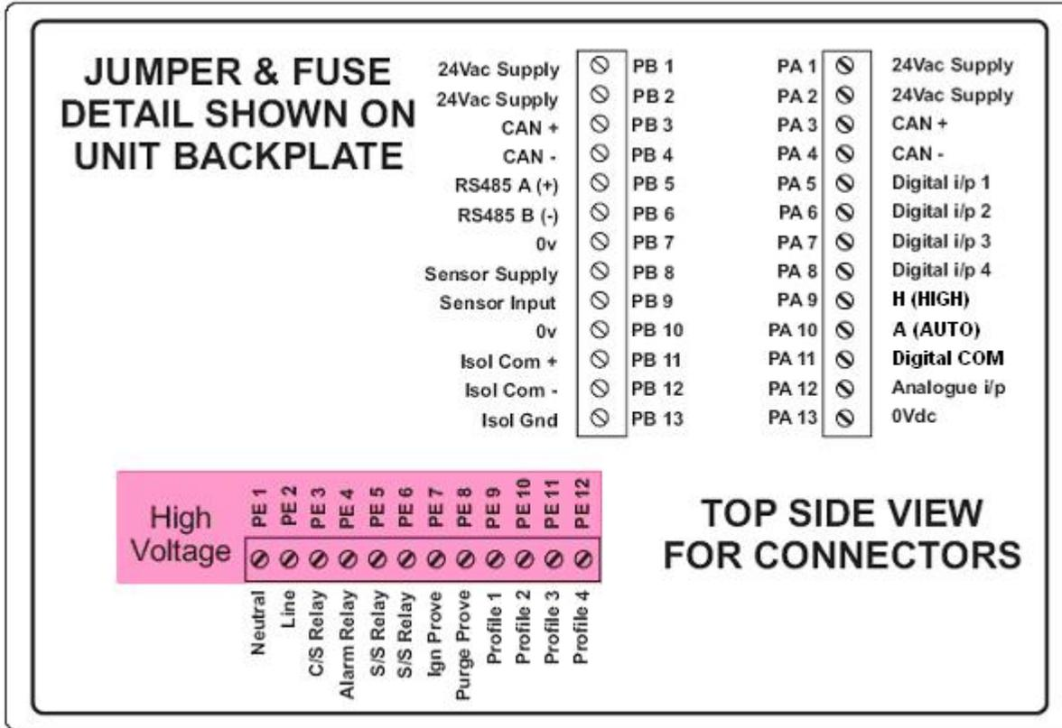
**Note: All wiring to terminals “PA & PB” are low voltage and must be braided shielded wire per table 2.6.1A of Fireye Bulletin PPC-6001. Wiring to terminals “PE” are line voltage. The maximum wire size is 16AWG (19.3mm) for all terminals.**
