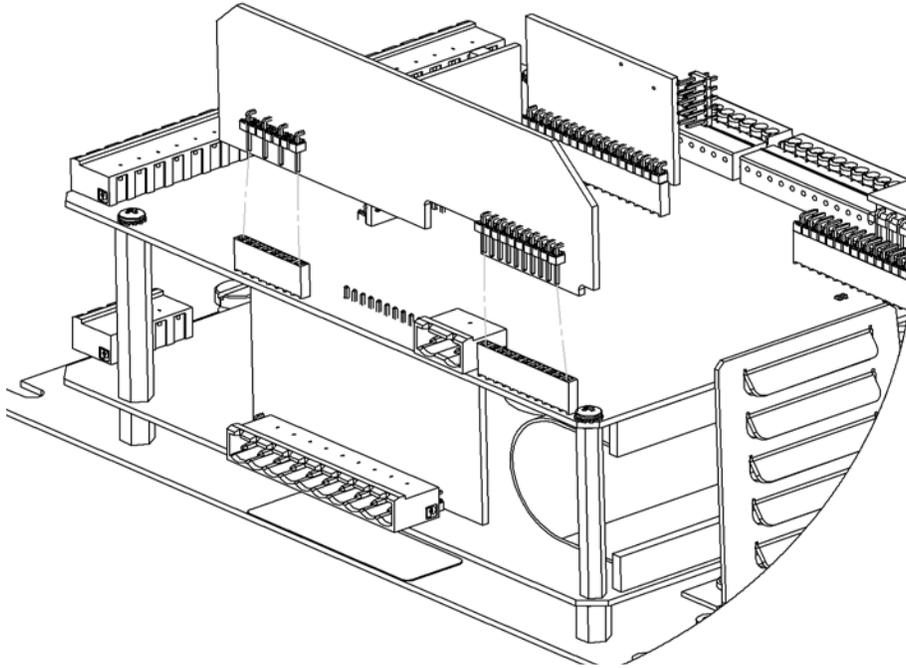
8. Re-install cover over NXF4000 until screws are contacted against standoffs.
