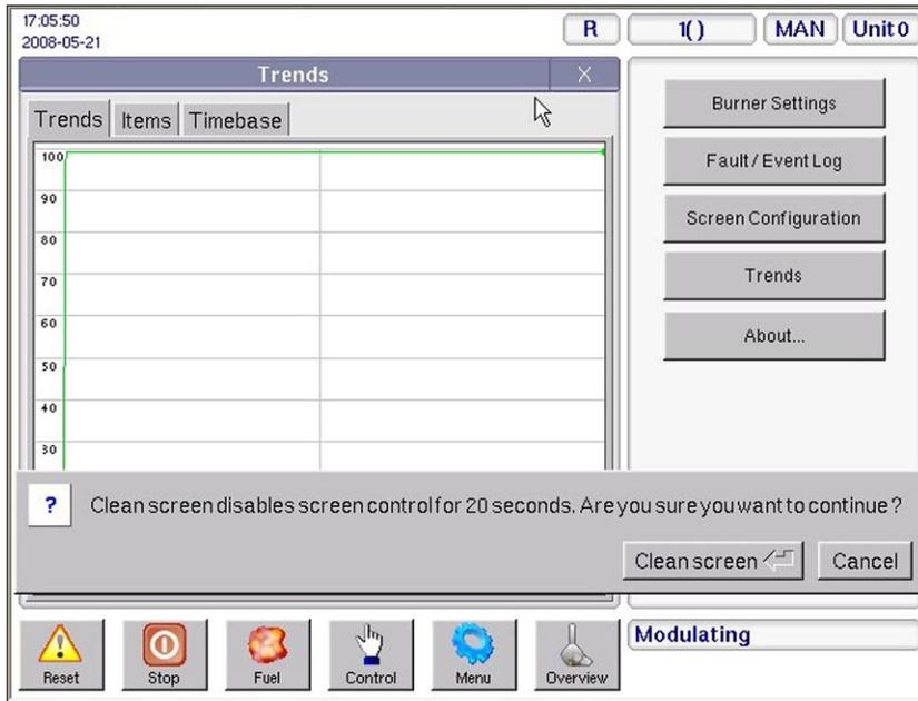
When cleaning the touchscreen ensure the correct LCD screen cleaner is used. Use of any other cleaning fluid or water may damage the screen.
