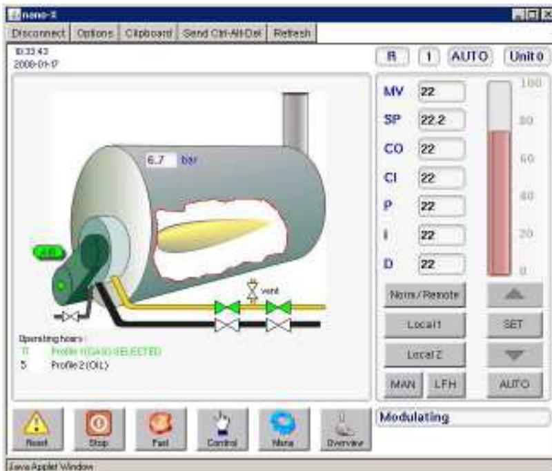
If the burner is firing, then the modulation percentage will be displayed on the vertical bar graph (0-100%), as well as numerically inside the box..
