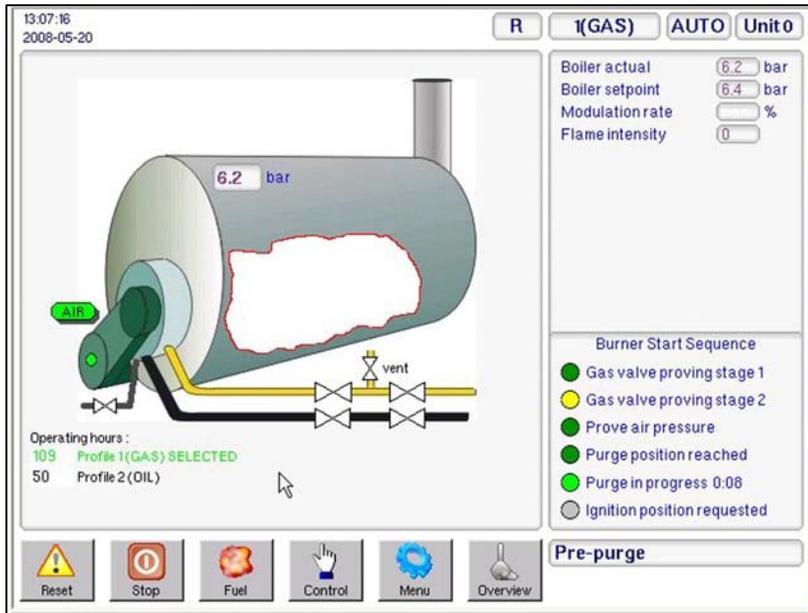
While the burner is changing 'status' the bottom-right one sixth of the display is used to provide a graphical indication of changing status.
