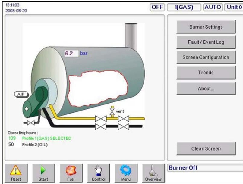
Using the buttons available after pressing the **Menu** button will generate a new pop-up window in the left hand area of the screen.
