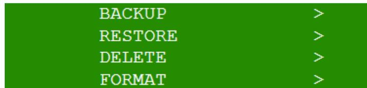
With the NXD410TS, the menu will jump to the SD CARD OPS SETUP line of the home screen automatically when the SD card is inserted. The arrows can also be used to access this menu if the card is already inserted. From this menu, choose the desired action: BACKUP, RESTORE, DELETE or FORMAT.
