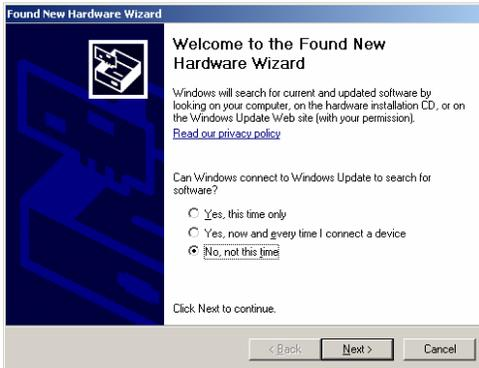
**#1.** Plug the UC485 into an available USB port on your Windows compatible computer or connected hub. The screen above appears, telling you that there is a new device plugged into the USB bus. Click on *No, not this time*, then the **Next>** button.
