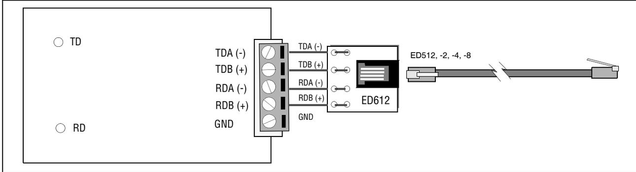
2. Connect the ED612 (RJ12 female connector provided with the UC485) to terminals TD(A), TD(B), RD(A), and RD(B) on the UC485
