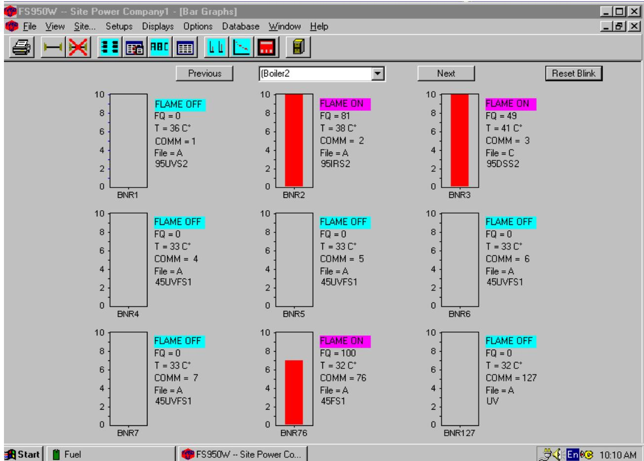
The Flame Quality is depicted as a value from 0 to 100. The scanner description, current file, Current Temperature and Comm Address are also shown.
