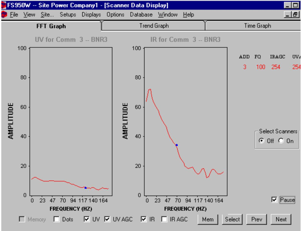
*Note: In the above figure, the “dot” on the UV FFT curve indicates that a target frequency of 117 Hz. has been programmed into the InSight scanner for the ultraviolet sensor. The “dot” on the IR FFT curve indicates that a target frequency of 70 Hz. has been programmed into the InSight scanner for the infrared sensor.*
