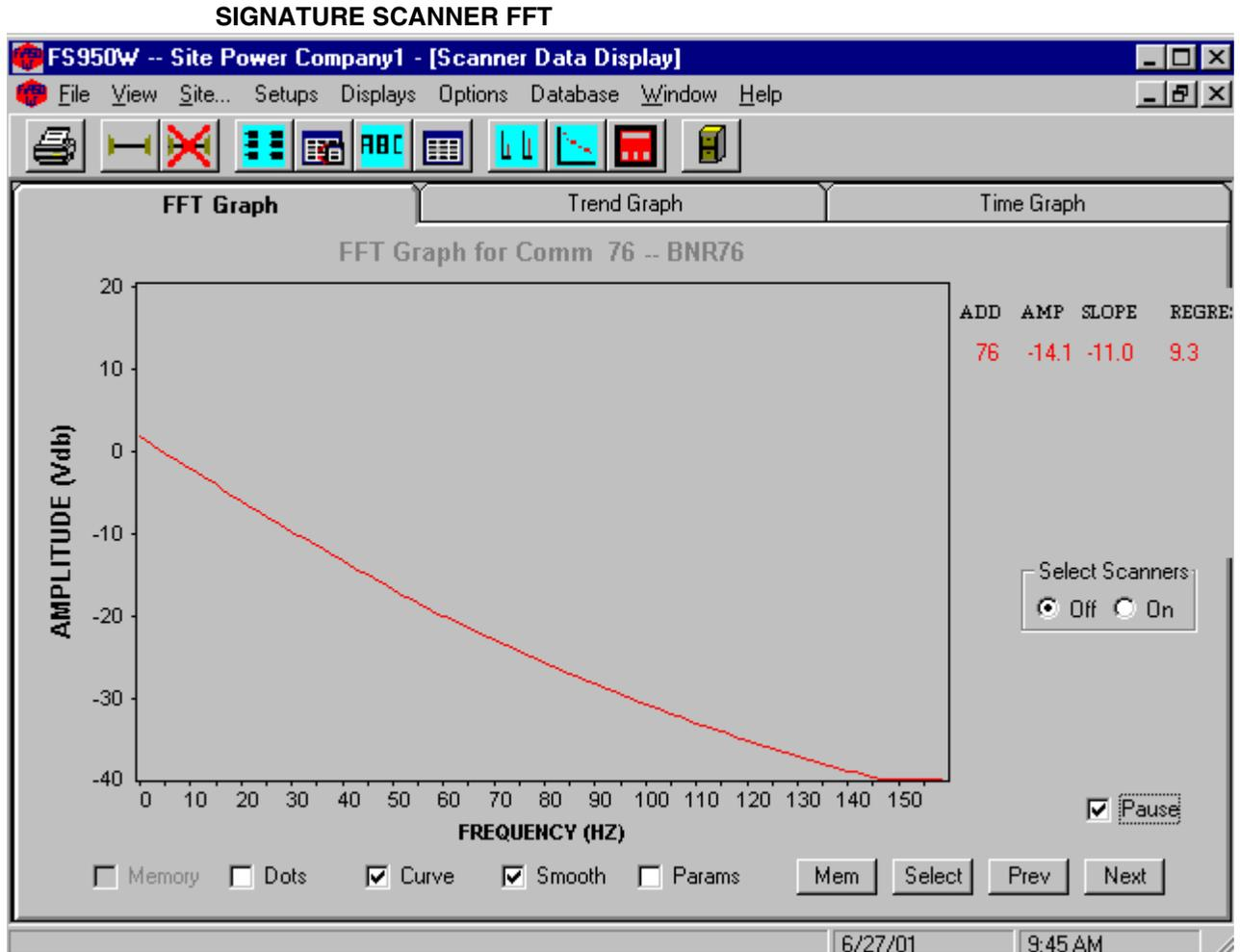
The Signature Scanner uses a 256 point Fast Fourier Transform to analyze the data from the target flame. The FFT screen contains the graphic representation of those points.
