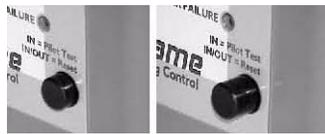
In the pilot test mode, the sbSeries will hold the sequence once the pilot flame is established and prevents energizing the main valve (terminal 5).
