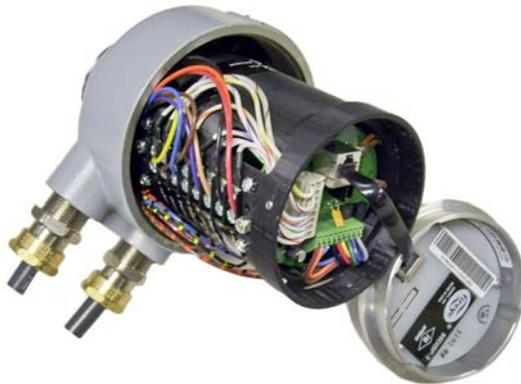
4. Connect the new Display cable to the new Display and to the scanner electronics assembly.
