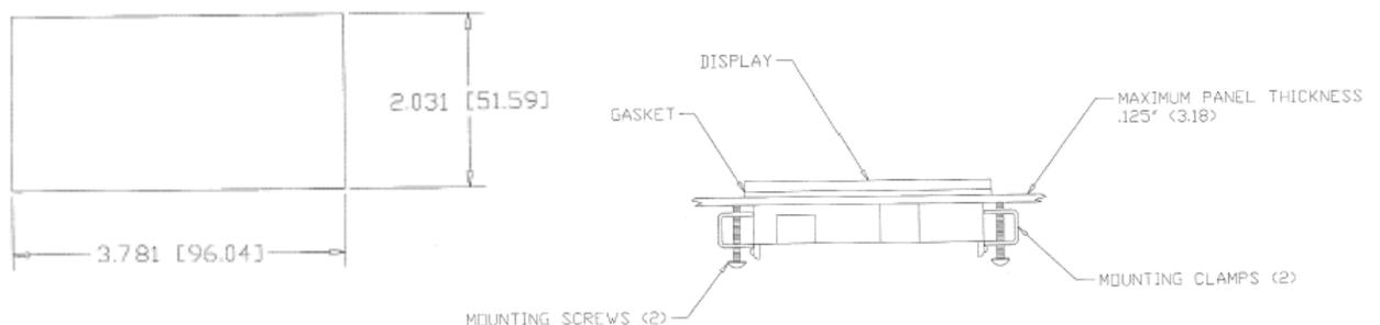
To install the BLL510 or BLV512 display module using the remote mounting kit (129-178-4 and -8):
