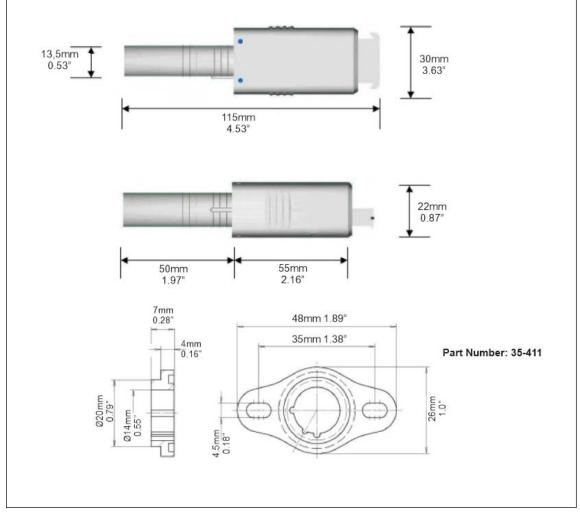
Use two #8-32 PAN or M4 PAN screws to secure flange to mounting surface
