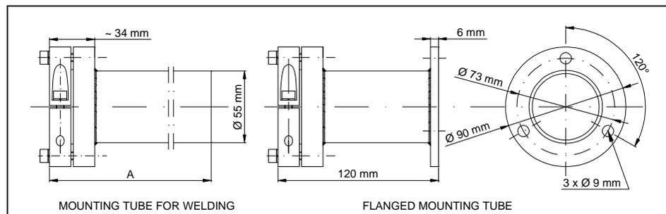
For fixing the pilot burner to a burner plate there are two types of mounting tubes available (material: carbon steel), offered as an optional accessory and to be ordered separately (see Fig. 2):
