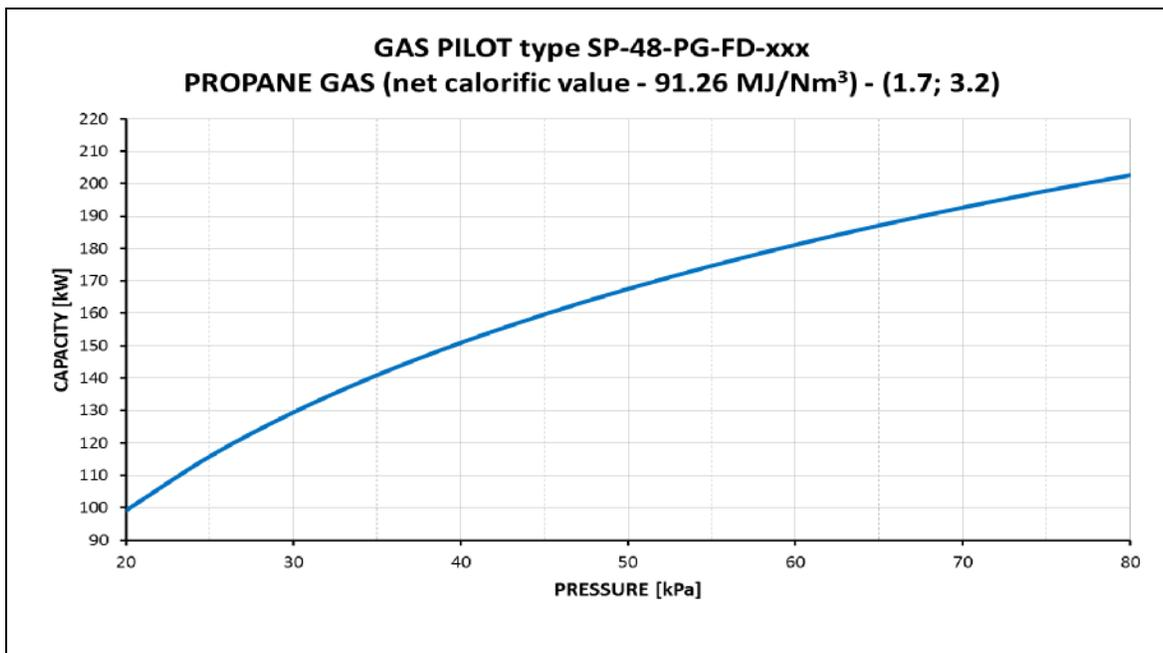
**Remark:** The real measured capacity may differ by  $\pm 5\%$  depending on a particular pilot and measurement conditions
