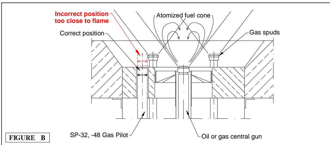
**Fig. A** Typical for power & utility boilers, industrial heaters - shows position of **SP-32** and **SP-48** Gas Igniter operating as an intermittent (light-off) on a sample single gun main burner, oil or gas fired, vertical or horizontal mounting.
