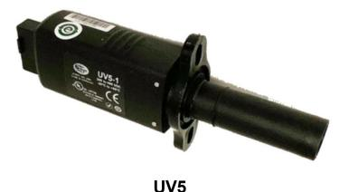
The UV1AL, UV90L and UV5 ultra-violet flame scanners are non-self-checking and should be applied only to burners that cycle a minimum of once per 24 hours. Cycling the burner once every 24 hours of continuous run time can be implemented into the BMS PLC programming to satisfy this requirement.
