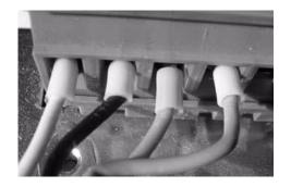
All cabling that is required to operate at above 50V must be multi-strand single core, PVC insulated, at least 0.5 mm<sup>2</sup> (20 AWG) and should meet the requirements of I.E.C. 227 or I.E.C. 225.
