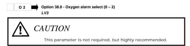
Option parameter 38.0 is only available when option 30.5 (oxygen input select) is not set to zero and the optional oxygen probe interface unit is connected.
