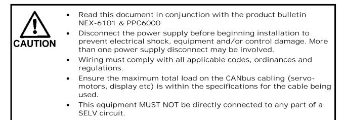
WIRING INSTALLATION MUST BE CARRIED OUT BY A COMPETENT ELECTRICIAN AND IS SUBJECT TO I.E.E. WIRING REGULATIONS (BS 7671:1992) AND/OR LOCAL STANDARDS, WHICH MAY PREVAIL.
