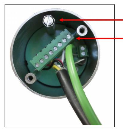
Calibration port. M4 female connector required
