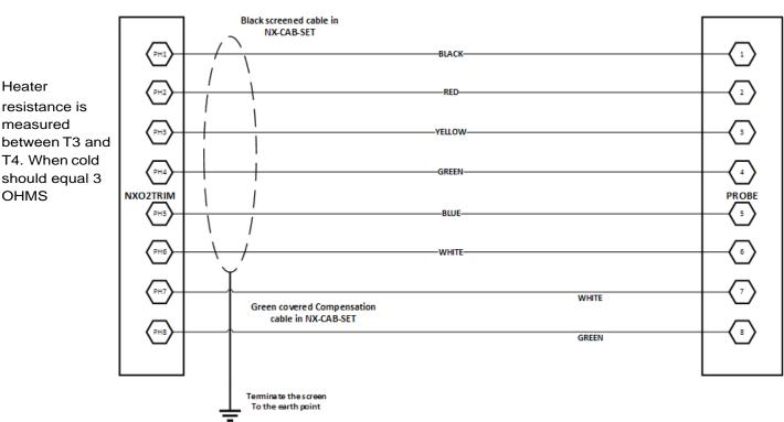
No screen connection at the probe. Trim the screen back to the outer insulation.
