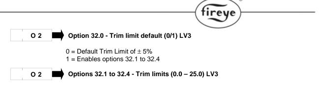
Option 32.0 is only available if option 30.5 (oxygen input function) has been set for closed loop oxygen trim.
