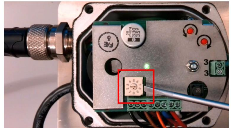
**For the exercise, check that the AIR servo is addressed to 1 and that the GAS servo is addressed to 2.**
