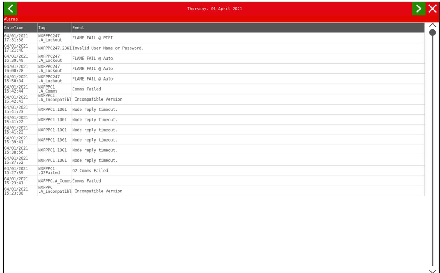
The screenshot displays the 'Alarms' interface on a touchscreen. At the top, there is a red header bar with a back arrow on the left, the date 'Thursday, 01 April 2021' in the center, and a close 'X' button on the right. Below the header is a table with three columns: 'DateTime', 'Tag', and 'Event'. The table contains 16 rows of alarm data. A vertical scrollbar is visible on the right side of the table.
