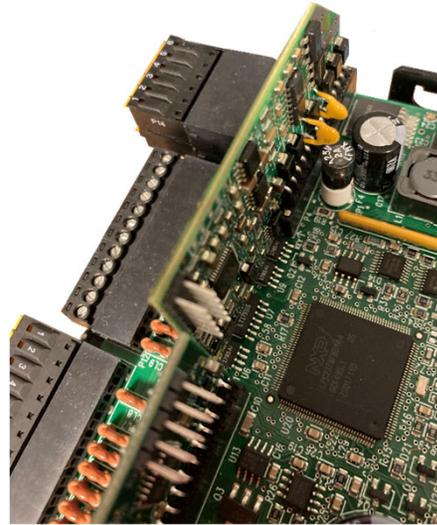
**For the exercise, power down the NXF4000 and disconnect each terminal block. Remove the plastic cover and find the NXCESVFD and the NXCESUV/NXCESIR amplifier cards. Remove and replace each card, then replace cover and terminal blocks.**
