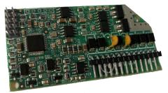
The NXCESVFD offers interfaces for up to two VFDs with either encoder feedback or with 4-20mA feedback from the VFD. The analog outputs from any unused channels can be used as user-assignable analog outputs.
