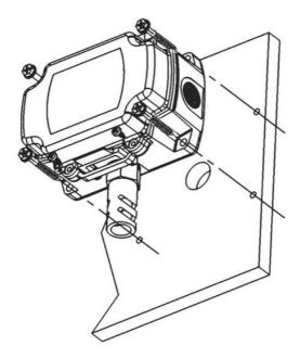
FXIATS-140 temperature transmitter installation
