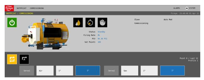
**NXF4000:** Once the burner on/off switch is set, the burner sequence will start and p01 can be commissioned.
