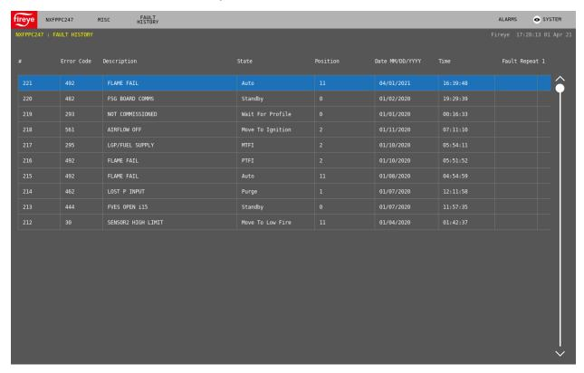
The NXTSD507HD and NXTSD512HD also captures alarms and system events locally. System events are abnormal occurrences such as communication loss, invalid password and similar. This allows more alarms to be retained than the NXF4000 and PPC4000 limit of the previous ten. Choose ALARMS  $\rightarrow$  ACTIVE to see the currently active alarms.
