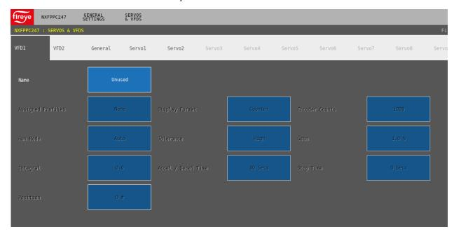
To enable the VFD for use, a name must be selected for the VFD. All the same names are available as with the servos and the same rules apply (at least one servo or VFD must be named AIR).
