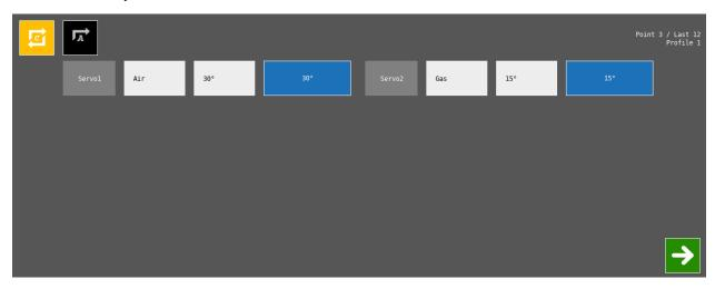
Since the gas regulator has been set already to make rate at the high fire position (see previous step), set the gas servo position based upon where the turndown can be verified, either by a fuel flow meter or by clocking the meter. It is important to check that the expected turndown is being delivered.
