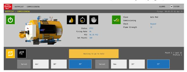
To confirm p02, exit check mode using the CHECK/RUN quick key and allow PTFI to complete. The NXF4000 will transition to MOVE TO LOW FIRE and allow p03 (first user defined point) to be commissioned. The NXTSD507HD and NXTSD512HD will both display a yellow banner MOVING TO POSITION P02 as the control purges.
