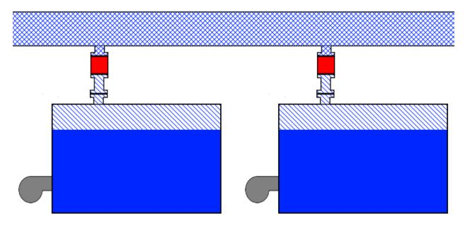
Boiler 1 is running and producing 6.89 Bar (100psi), which is going into the header. The non-return valve is keeping the steam out of boiler 2, which is not making any steam and is cold since it has been off for several days.
