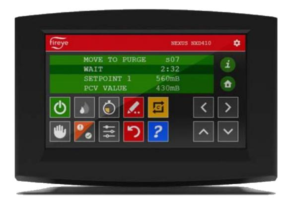
The NXD410TS display provides four lines of information. The active area of the display is highlighted on the second line. The four directional keys (located on the right-hand corner) are used to navigate through the menus and to update values. The next section shows the various symbols and their functions.
