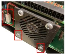
Remove connector and screws
