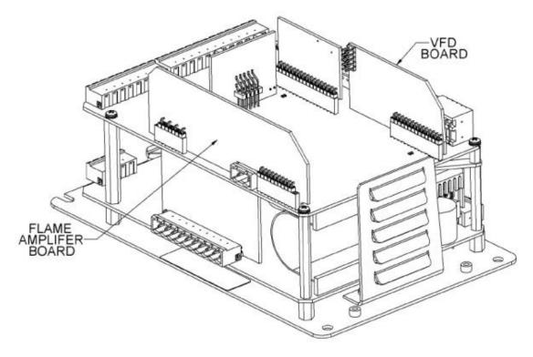
Diagram of NXF4000 with cover removed
