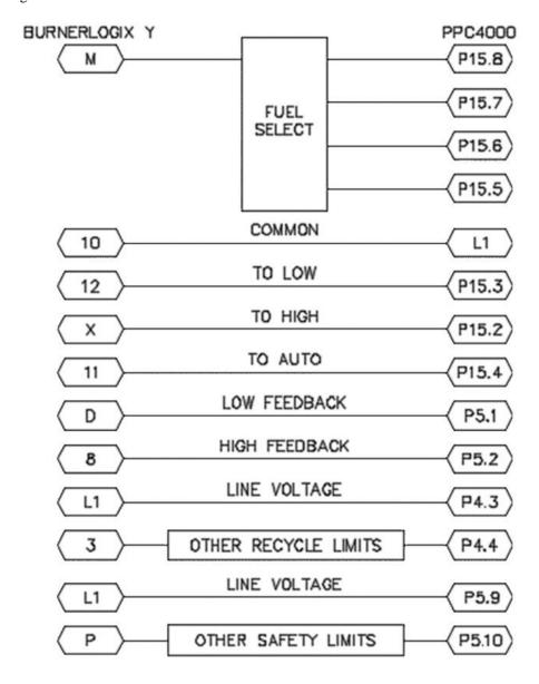
$Example\ wiring\ interface\ from\ Burner Logix\ to\ PPC 4000$
