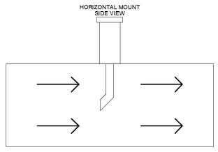
Alternate mounting when stack is horizontal (preferred)
