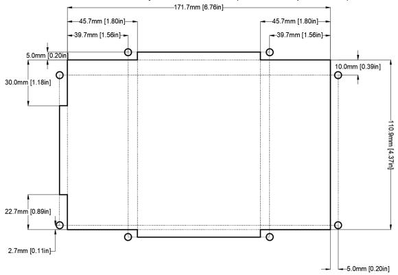
Holes are for M4x0.7 threaded posts with knurled-head thumb nuts (minimum clearance shown)
