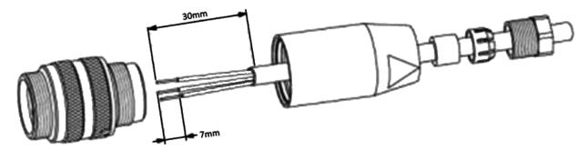
As shown above the cable strip length is specified at 30 mm (1.2 in) and each wire strip length is 7 mm (0.275 in).
