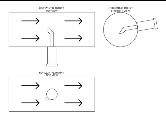
Alternate mounting when stack is horizontal (acceptable)
