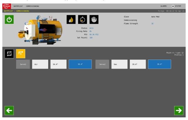
Once the burner is in the automatic state, use the LEFT and RIGHT quick keys to change which point is being adjusted. On the NXD410TS, these points will be referred to as a03...a23 instead of as p03...p23 while in this mode. Once the control has moved to the desired point the servo and VFD positions can be modified in the same manner as when commissioning. When finished adjusting, press the C-MODE or ADJUST RATIO quick key to return to automatic operation.
