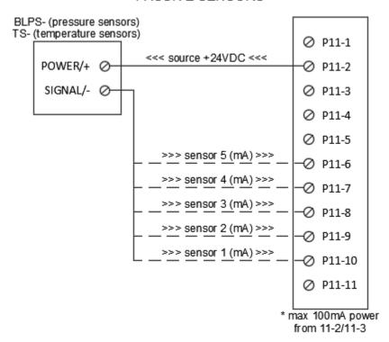
It is recommended that shielded cable is used to connect any sensor. Only ground the shield on one side of the connection to prevent ground loops.
