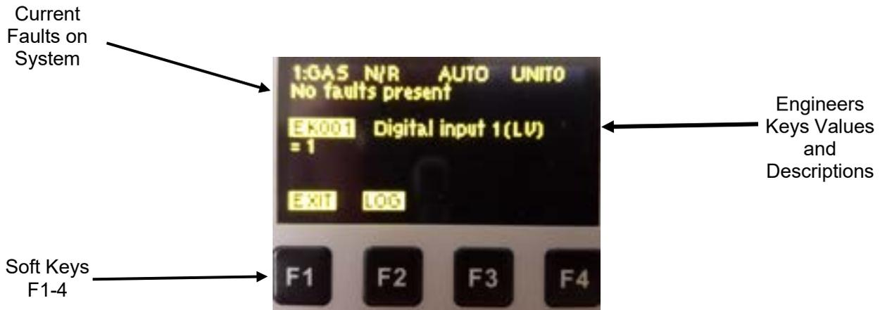
SEE Section 6 of Fireye Bulletin NEX-6101 or PPC6001 [Fault and Fault Finding] for Engineers Key Descriptions.
