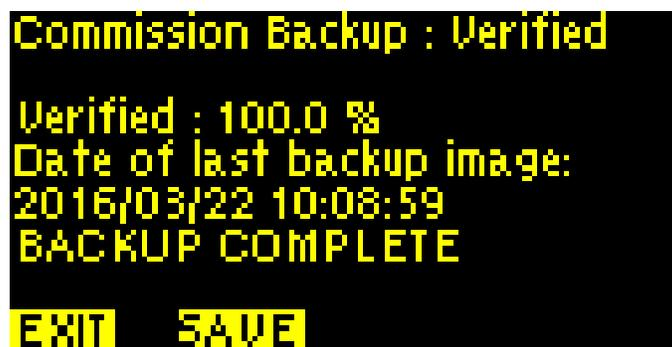
A screenshot of a device's backup status screen. The text is displayed in yellow on a black background. It reads: "Commission Backup : Verified", "Verified : 100.0 %", "Date of last backup image:", "2016/03/22 10:08:59", "BACKUP COMPLETE", and at the bottom, "EXIT SAVE".
