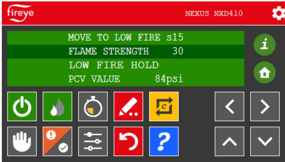
Selecting the low fire key modulates to low fire hold.
