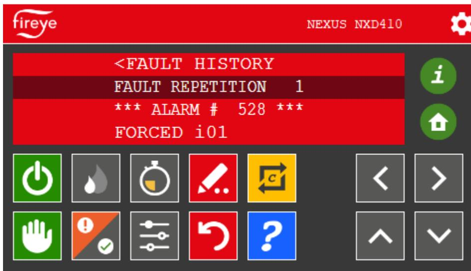
A Lockout occurred on Digital Input 1. It is the 528<sup>th</sup> lockout.
