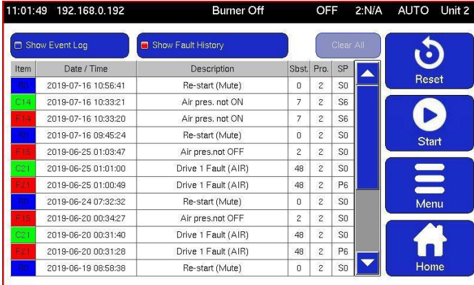
Example after tapping Menu > Fault/Event Log
