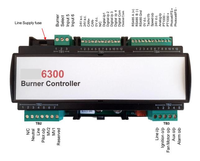
Each terminal set has a removable block to make wiring a little easier. The terminal blocks must be pushed fully home to ensure reliable operation.
