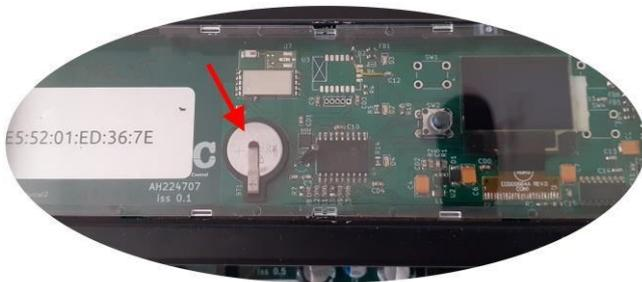
Access to the battery is by removal of the top cover by prying it off like this...
