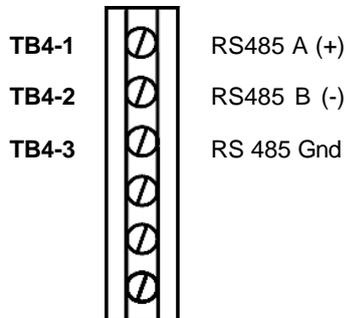
The RS485 cabling **MUST** be overall 'braid' screened, PVC insulated, 3-core of 0.25 mm<sup>2</sup> (AWG 24) wire. The rules for ELV circuits, defined in 2.1.4, apply.
