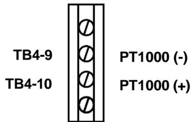
The sensor cabling **MUST** be overall **'braid' screened** PVC insulated 0.25 mm<sup>2</sup> (AWG 24).
