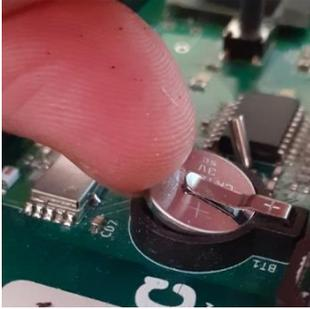
When the battery has been removed, the replacement battery can be inserted into the holder. Insert the battery into the holder at an angle with the flat side facing upward, as shown in the following picture, and then push into place in the direction of the arrow.
