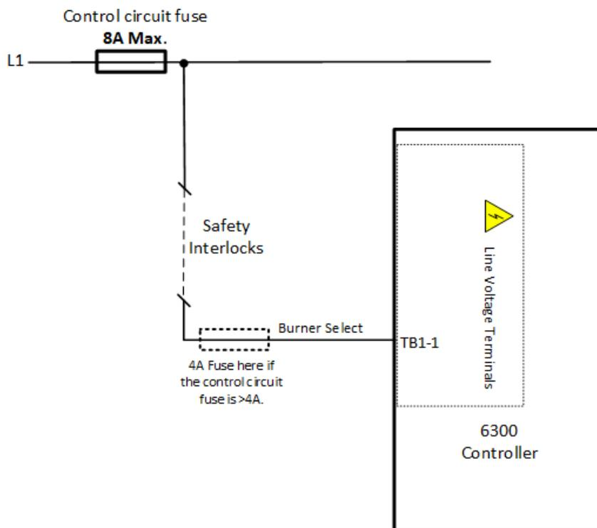
Connect the Burner select input to the devices upstream in the safety interlock chain, using multi-strand, single core, PVC insulated 0.5 mm<sup>2</sup> (AWG 20) wire.
