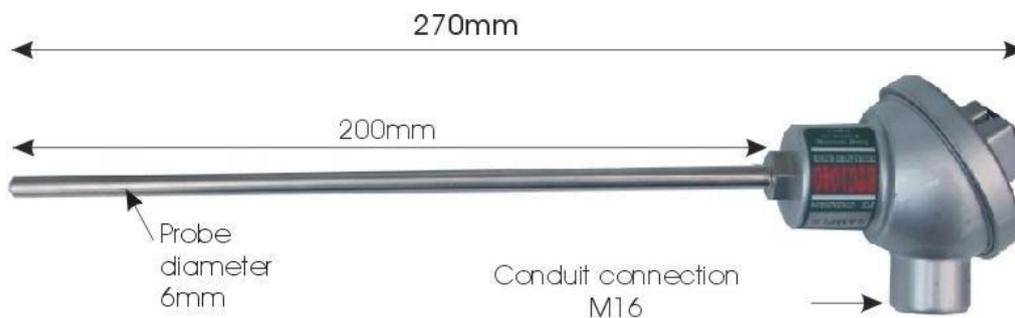
The temperature sensor has a protection level of IP65 if suitable conduit glands are used, and it can be mounted in any attitude. It has been designed for mounting into a well, or pocket, that has been inserted into the boiler shell. When choosing the position of the well, make sure that the sensor will operate within its environmental specifications, and that the position will allow measurements and subsequent control actions to be correlated to other devices e.g., auxiliary safety stats.
