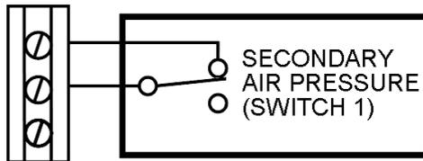
Connect these terminals to the appropriate terminals on the burner's air pressure switch.
