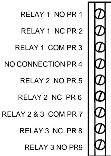
Fuses not exceeding 4 A must protect all relay outputs. Fit a 4 A fuse to the Burner Panel Supply, relay common or, where the total current exceeds 4 A, fit a separate fuse on each relay COM terminal to achieve this.
