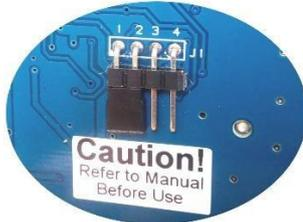
2. In this setting mode the position feedback value will indicate zero degrees on the HMI.
