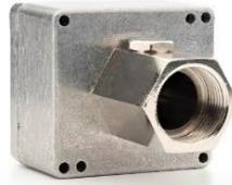
Mount the flame detector to the burner by way of a 1" NPT thread to a sighting tube on the burner front. There is provision for an air purge/cooling connection on the hexagonal section of the body.
