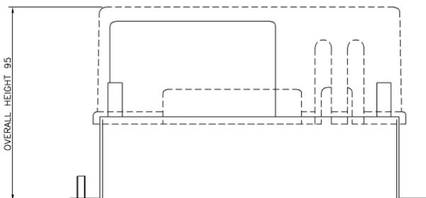
The device MUST be installation inside a burner control cabinet. The cabinet should have a minimum protection level of IP54.
