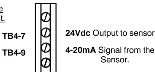
The sensor cabling MUST be overall **‘braid’ screened** PVC insulated 0.25 mm<sup>2</sup> (AWG 24) (number of cores as required by the relevant sensor).
