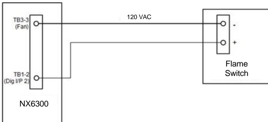
Set option parameter 13.0 to a value of 1 for this mode of flame detection.
