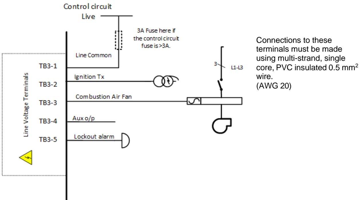
**Fuses not exceeding 3 A must protect all relay outputs from the TB3 terminal block.**
