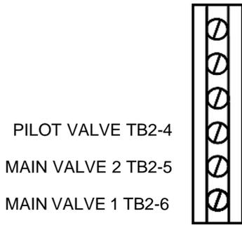
The Burner Select input supplies the power to the fuel valve energizing circuits.
