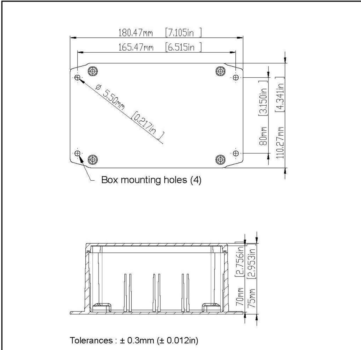
If you use suitable conduit glands, the optional NXO2TRIM Oxygen Probe Interface unit has a protection level of IP65. You can mount it in any orientation, either inside or outside a control cabinet.
