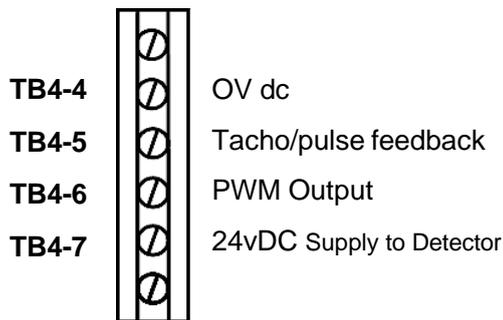
All speed and feedback cabling MUST be overall 'braid' screened, PVC insulated, multi-core of 0.25 mm<sup>2</sup> (AWG 24) wire. The rules for ELV circuits, defined in 2.1.4, apply.
