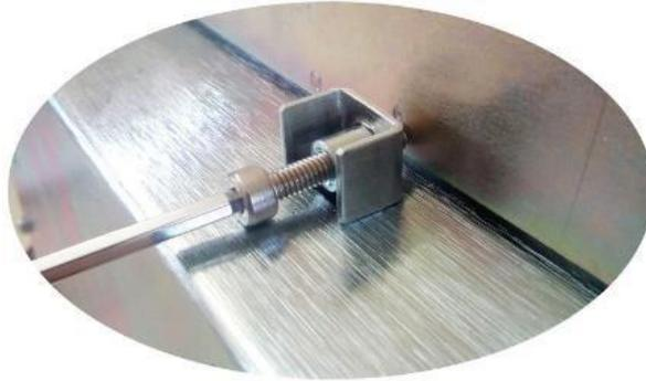
Tighten until the fascia plate of the HMI is tight to the enclosure door forming an IP65 seal to the door front surface.
