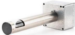
Mounting the flame detector to the burner is by way of a clamp ring around the sight tube. If there is any doubt that the burner casing is not a good electrical Earth, then the clamp ring must be connected to electrical ‘Earth’ using suitable cable.
