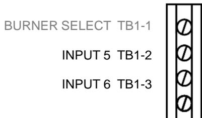
Connect these inputs using multi-strand single core PVC insulated 0.5 mm<sup>2</sup> (AWG 20) wire.
