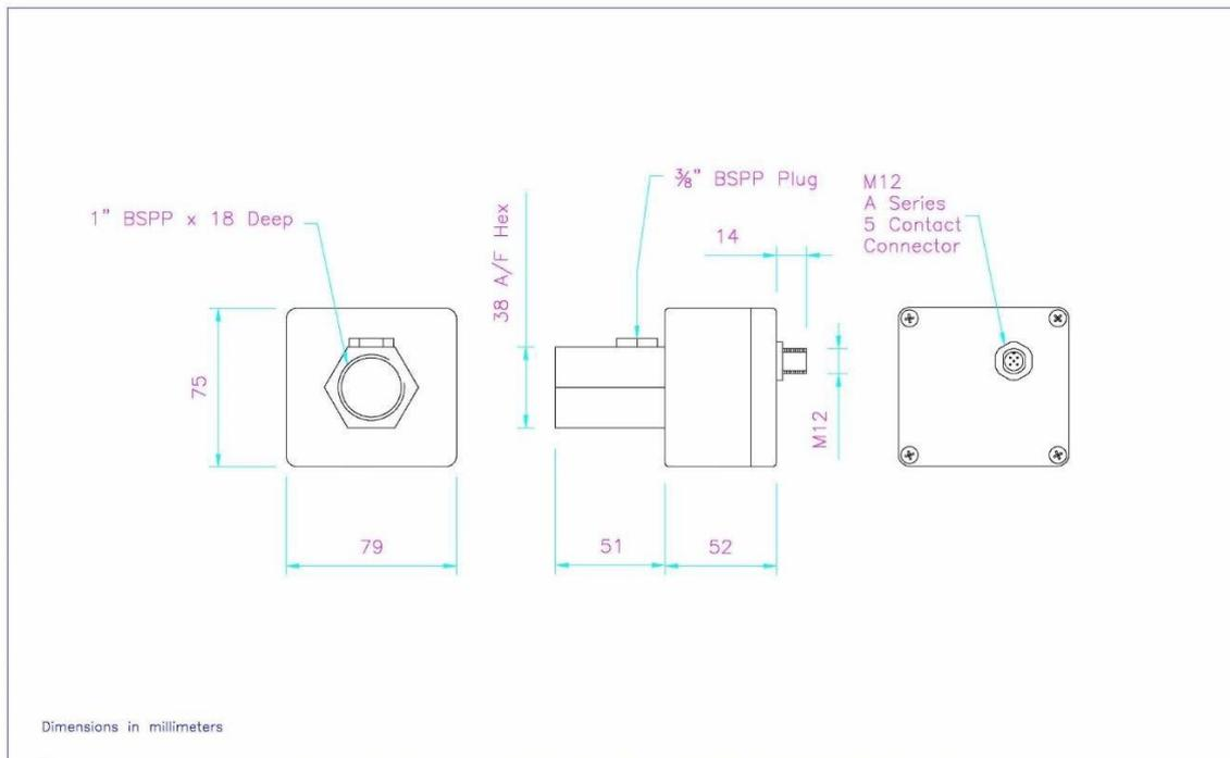
Electrical connection is by way of a 12mm plug and socket on the square section of the body. The ambient operating temperature range for this device is -20 to 60 °C (-4 to 140 °F).
