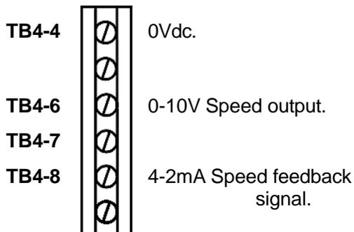
All speed and feedback cabling MUST be overall 'braid' screened, PVC insulated, multi-core of 0.25 (AWG 24) mm<sup>2</sup> wire. The rules for ELV circuits, defined in 2.1.4, apply.
