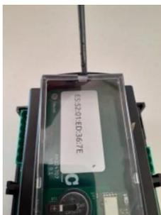
With the cover removed the battery can be removed out of the holder with a non-conducting tool or a fingernail like this....
