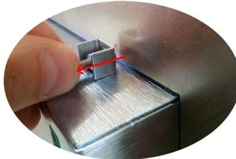
Then the hexagon cap head clamp screws (3mm AF) are tightened evenly.
