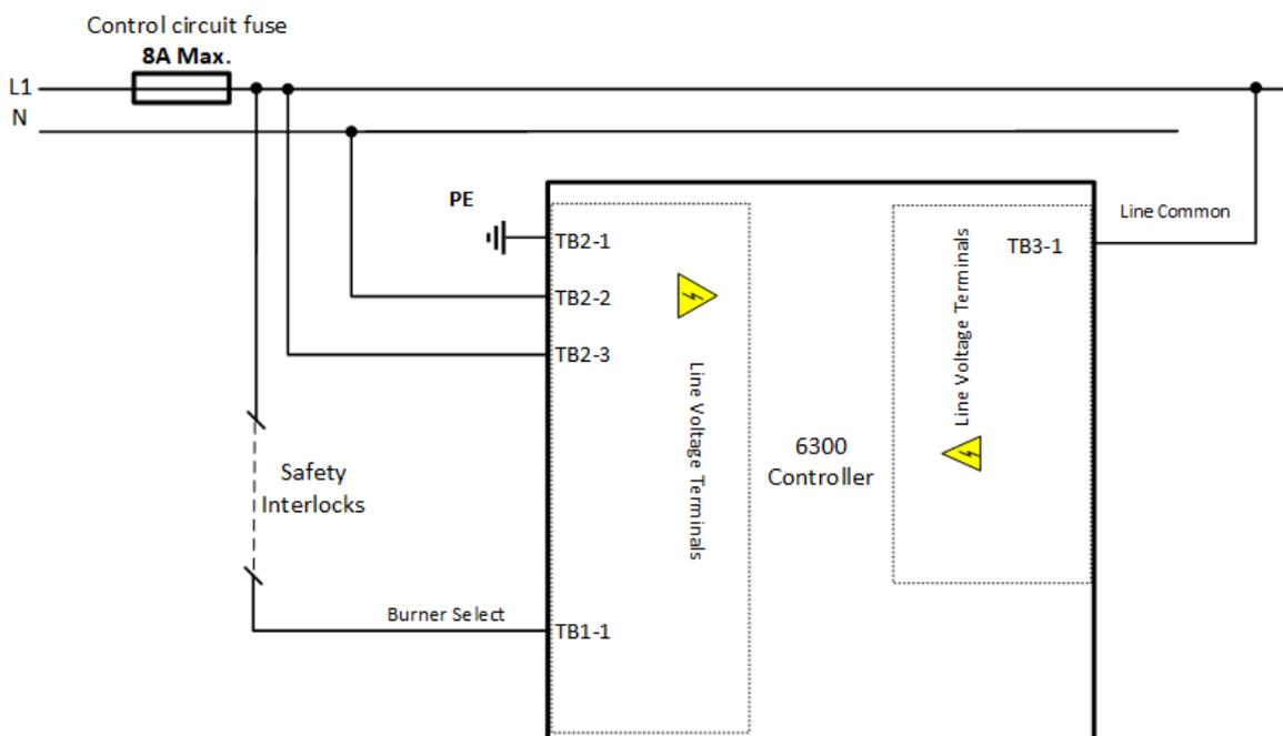
**NOTE:** If a control circuit fuse greater than 4 A is required, then the feeds to TB1-1 and TB3-1 must be individually fused, to protect the output relay contacts from 'welding'. More details are given in the next two pages.
