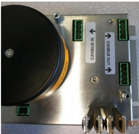
There is a 2-way terminal block for the live voltage connection (bottom-left).
