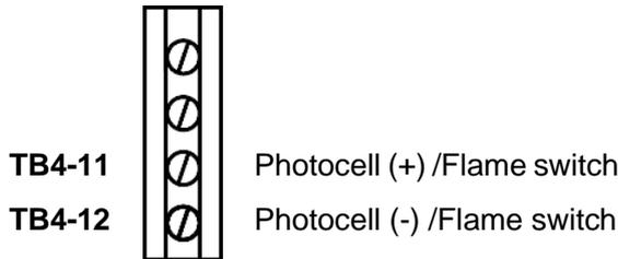
Install and wire the photocell or VFC according to the instructions supplied with the sensor device. The flame sensor **MUST** be connected using multi-strand overall 'braid' screened, PVC insulated, 2-core of 0.25 mm<sup>2</sup> (AWG 24) wire.
