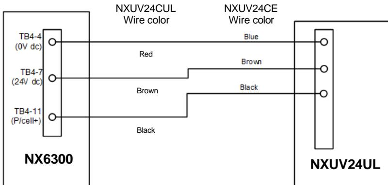
The standard cable for the KLC device is not screened. Where the distance between the KLC device and the NX6300 is greater than 600mm, (2 ft.) then screened cable must be used to extend the cable length using multi-strand overall 'braid' screened, PVC insulated, 3-core of 0.25 mm<sup>2</sup> (AWG 24) wire.
