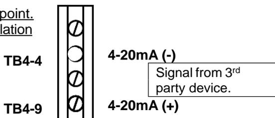
Connect the cable ‘braid’ screen to earth at an Earthed DIN terminal in the panel. Ensure that the screen covers the signal wires until 30mm from the TB4 terminals.
