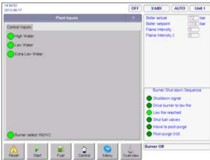
Example after tapping Menu > Plant Inputs
