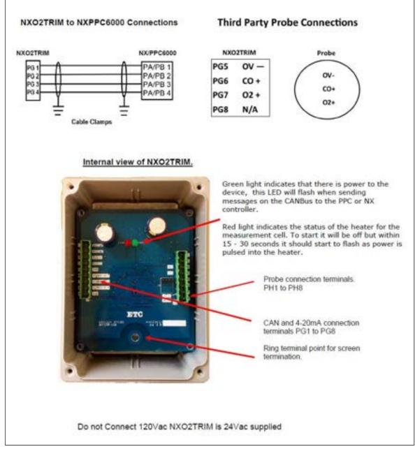
NOTE: 4-20mA  $O_2$  input from non-Fireye  $O_2$  probe. See sections 30.1 and 30.2
