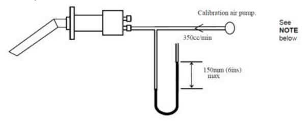
If the pressure is 150mm (6ins) water gauge or more the filter must be replaced.
