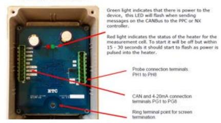
NOTE: 4-20mA O2 input from non-Fireye O2 probe. See sections 30.1 and 30.2
