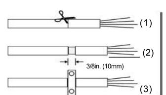
The cable should be prepared by cutting around the outer insulation, taking care not to damage the screen (1).
