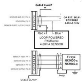
The pressure/temperature cabling MUST be overall braided shielded (screened) PVC insulated 24 AWG (7/0.2mm) (number of cores as required by the relevant sensor). Since this cable may be run adjacent to, and/or in the same conduit as high voltage wiring, its voltage rating must exceed the maximum voltage carried by any other cable connected to the control or run in the same conduit.
