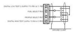
These inputs MUST be connected using multi-strand overall braided shielded (screened) 2, 3 or 4 core (as required) PVC insulated 24 AWG (7/0.2mm) wire. Since this cable may be run in conduit with high voltage wiring, its voltage rating must exceed the maximum voltage carried by any other cable connected to the control or run in the same conduit.
