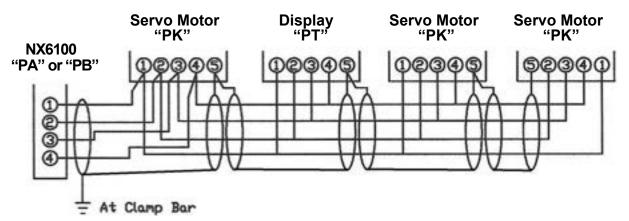
NOTE: See Page 34 for recommended wire. No "or equals" is provided Remove and replace with below. See CANbus wire chart for approved cable No "or equals" or substitutions.
