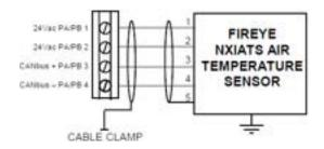
The system allows direct connection of an FIREYE inlet temperature sensor. The unit is connected via CANbus similar to the servo-motors and display, using overall screened 4 conductor (core) 24 AWG (7/0.2mm) PVC insulated cable. Since this cable is to be run adjacent to, and/or in the same conduit as high voltage wiring, its voltage rating must exceed the maximum voltage carried by any other cable connected to the control or run in the same conduit. See Sections 2.6.1 & 2.6.2.
