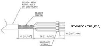
2) Clamp the braided screen between the lid and the clamp plate with the wire tails protruding from the 'D' cutout as shown below. Fix the clamp plate into the sensor cap using the screws provided. **This connection must be made for proper operation.**
