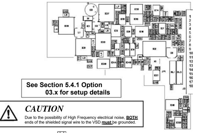
4-20mA Output Channel 1 – PZ 1 4-20mA Output Channel 1 + PZ 2 4-20mA Output Channel 2 – PZ 3 4-20mA Output Channel 2 + PZ 4 4-20mA Output Channel 3 – PZ 5 4-20mA Output Channel 3 + PZ 6 Counter Input 1 PZ 7 +12Vdc PZ 8 Counter Input 2 PZ 9 +12Vdc PZ 10 Counter Input 3 PZ 11 Input Channel 1 - PZ 12 Input Channel 1 ± PZ13 Input Channel 2 + PZ14 Relay 7 common PZ 15 Relay 7 normally open PZ 16 Relay 8 common PZ 17 Relay 8 normally open PZ 18
