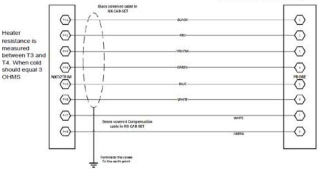
No screen connection at the probe. Trim the screen back to the outer insulation.
