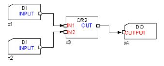
Briefly, this program will give a relay closure (digital output, DO) if either of the digital inputs (DI-1 or DI-2) is activated. These inputs could come from relay closures on other equipment.
