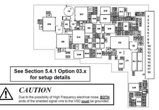
4-20mA Output Channel 1 ve PZ 1 4-20mA Output Channel 1 +ve PZ 2 4-20mA Output Channel 2 -ve PZ 3 4-20mA Output Channel 2 +ve PZ 4 4-20mA Output bChannel 3 -ve PZ 5 4-20mA ĺŻ Output Channel 3 +ve PZ 6 ۲Ż Counter Input 1 PZ 7 +12Vdc ĺŻ PZ 8 Counter Input 2 PZ 9 Z +12Vdc PZ 10 Counter Input C 3 PZ 11 Input Channel 1 -ve ĺŻ PZ 12 Input Channel 1 +ve & C 2 -ve PZ13 Input Channel 2 +ve PZ14 Relay 1 common ĺŻ PZ 15 Relay 1 normally open PZ 16 Relay 2 common PZ 17 Relay 2 normally open PZ 18
