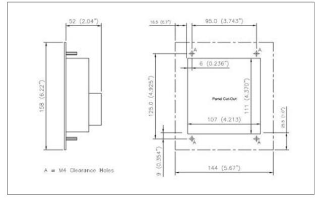
NOTE: Cut out dimensions of the NX6220, NX6330 and NX610 are slightly larger than the NX6110. Mounting holes are the same location as the NX6110, but not the NX610 (9 key) display. Cut out is approximately 5/16" larger vertically, 1/8" wider horizontally.
