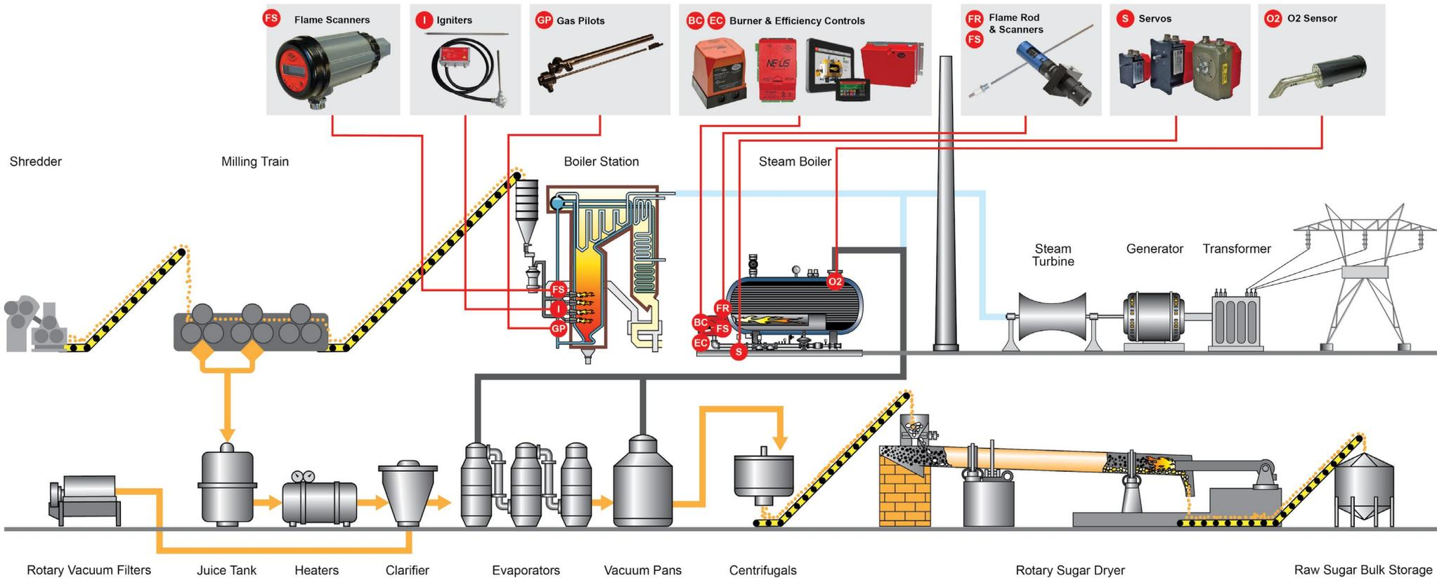
Flame safeguard and efficiency controls with Ultraviolet (UV) and Infrared (IR) flame scanners, flame rod, valve servomotors and O2 trim options.
