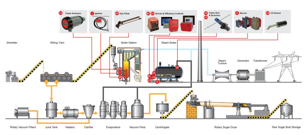
Flame safeguard and efficiency controls with Ultraviolet (UV) and Infrared (IR) flame scanners, flame rod, valve servomotors and O2 trim options.
