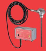
The SureFire II high-energy ignition system is used for direct spark ignition of most gas or liquid fuels used in oil or gas igniters or main burners. The high-energy ignition system is available in various versions. To ensure optimal operation, the first part of the ignition tip should always be in an ignitable fuel-air mixture, during all modes of operation.
