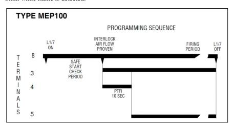
Terminal #5 is energized 3 seconds after flame is detected. Re-ignited PTFI on flame fail after Terminal 5 energized. Recycle on loss of interlock (air flow) after flame proven.
