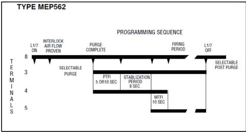
Pilot stabilization timing begins as soon as flame is proven. Lockout on loss of air flow (interlock circuit) after flame is proven. Lockout on flame fail.
