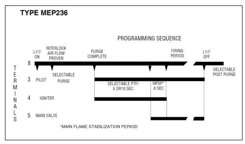
Terminal #5 is energized 3 seconds after the flame is detected.
