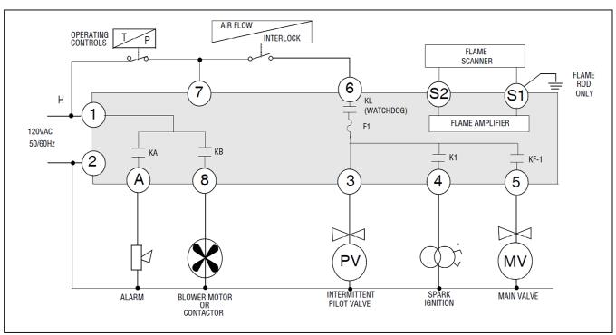
**FIGURE 8.** WIRING ARRANGEMENT FOR DIRECT SPARK IGNITED BURNERS, TWO STAGE OPERATION USING MEP100 AND MEP200 SERIES PROGRAMMERS
