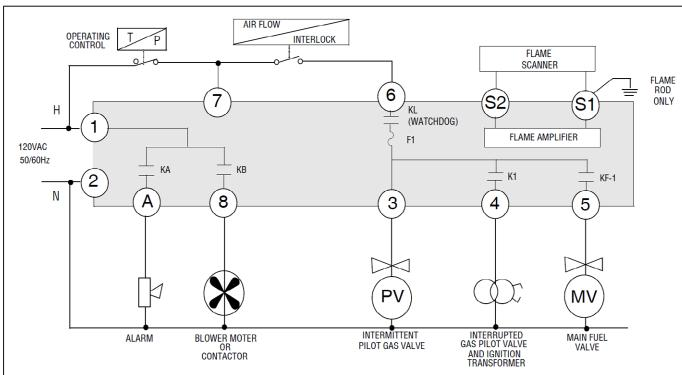
FIGURE 10. WIRING ARRANGEMENT FOR DIRECT SPARK IGNITED BURNERS AND INTERRUPTED IGNITION USING MEP500 SERIES PROGRAMMERS
