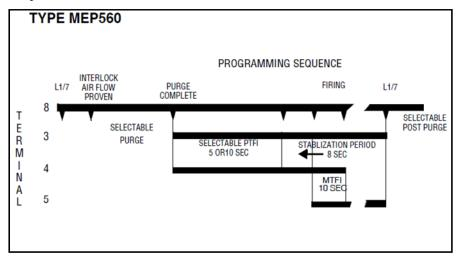
For the MEP560 and MEP562, after pilot flame is detected, the control enters an 8 second pilot stabilization period with Terminal 3 and Terminal 4 energized. At the expiration of the stabilization period, Terminal 5 is energized.
