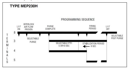
Pilot Stabilization timing begins as soon as flame is proven.
