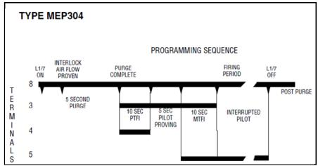
0 Second post purge on operating control open. 15 Second post purge on flame fail. Non-recycle operation on flame fail.
