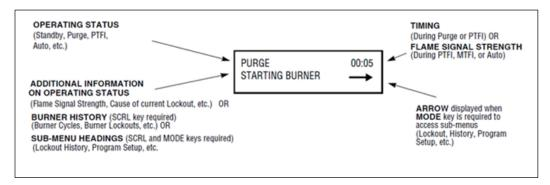
At any time the MicroM is powered, the SCRL key is used to scroll through and display the total number burner hours, burner cycles, burner lockouts and system hours on the bottom line of the ED510 display. The top line will continue to show the current run mode of the control (e.g. PURGE, AUTO, etc.) Following the historical information, the SCRL key will display three (3) sub-menus providing the following information and/or functions:
