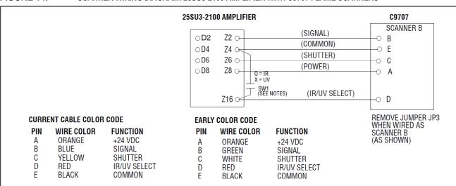
**IMPORTANT NOTE:** THIS SCHEMATIC IS TO BE USED ONLY WITH 25SU3-2100, OR WITH 25SU3-**2000** ENGINEERING CODE 32 OR HIGHER. THE ENGINEERING CODE WILL APPEAR WITH THE DATE CODE STAMPED ON THE REAR OF THE FACE PLATE (I.E. 9625-32). CONSULT FACTORY BEFORE USING C9707 SCANNER WITH AN AMPLIFIER WITH AN ENGINEERING CODE OF 30 OR EARLIER. DAMAGE COULD OCCUR TO THE SCANNER.
