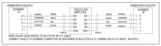
FIGURE 10. SCANNER WIRING DIAGRAM: 25SU3-2100 AMPLIFIER 19UVPS/45RM1, 45RM2 SCANNER WIRING COMBINATIONS1.2.3
