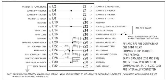
FIGURE 8. POWER WIRING DIAGRAM: 60-2470 24VDC POWER SUPPLY AND THREE 25SU3-2100 AMPLIFIERS
