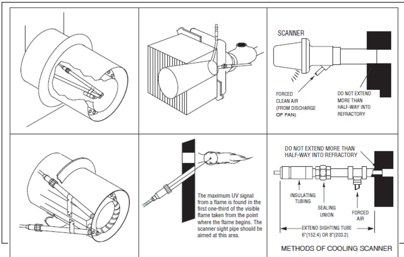
Self-checking ultraviolet scanners are used in applications where burner firing operation is continuous or where the burner is on for long periods of time without recycling. In addition, ultraviolet self-checking systems are mandatory in many locations.
