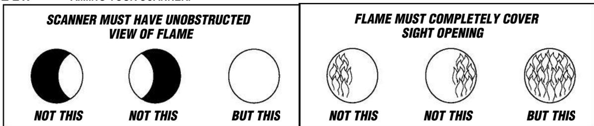
5. Smoke or unburned combustion gases absorb ultraviolet energy. On installations with negative pressure combustion chambers, a small hole drilled in the UV1A, UV2 sight pipe keeps the pipe clean and free from smoke. For positive pressure furnaces, provide clean air to pressurize the sight pipe, if necessary.
