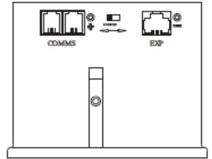
**FIGURE 31. 4-20mA TEST JACKS**
