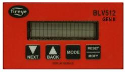
The NEXT key is used to scroll down through the various menus and is also used to increment the value when in the modify mode. The BACK key is used to scroll up through the menus and is also used to decrement the value when in the modify mode. The MODE key is used to enter a sub-menu when the displayed item indicates a sub-menu with a right facing arrow and to exit the sub-menu and move on to the next main menu item.
