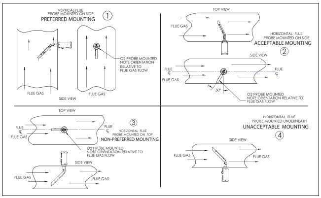
The vertical center line of the flange shown on the drawing should correspond to the gas flow direction. 6 stainless steel M6 x 20mm long socket cap screws are provided for probe or cover attachment.
