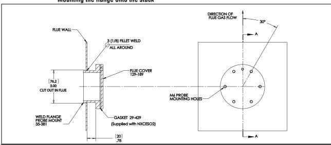
The probe flange temperature must be maintained at the temperature of the flue wall by repacking or adding lagging, which may have been removed to mount the probe. Sulfate condensation will occur if the flue wall of oil fired boiler falls below approximately 266°F (130°C). The sulfate problem does not occur in gas fired installations, but vapor may cause problems due to condensation if the temperature of the flue gas falls below 212°F (100°C).
