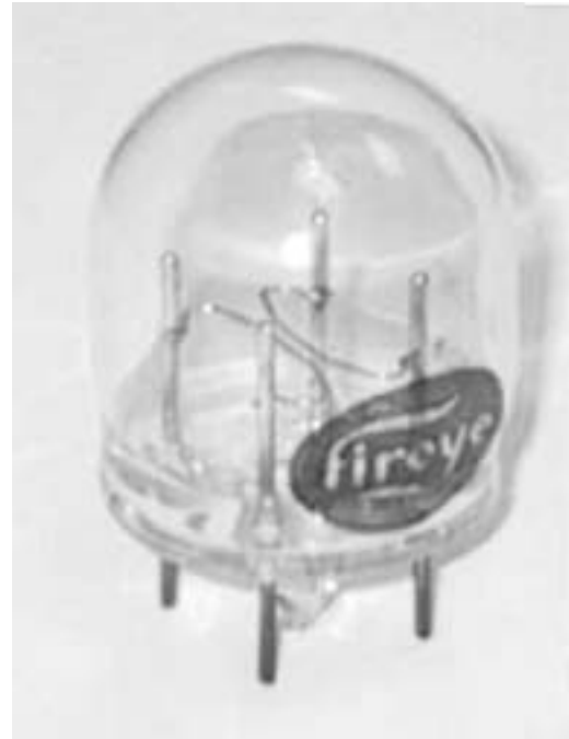
Fig. 10 UV radiation detection tube. Fireye part no: 4-320
