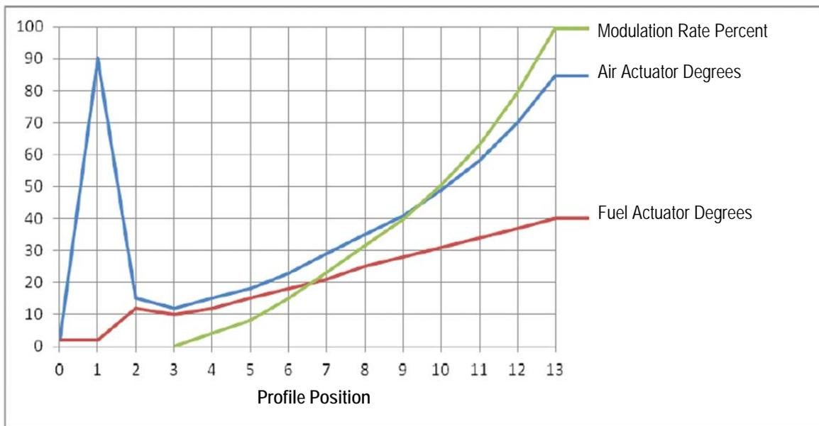
Graph 2 shows the same commissioned actuator positions for both the AIR and FUEL servos as shown graph 1 but with the FUEL actuator used as the master because a VFD is used. Notice how different the modulation curve appears. Because the FUEL's p03 position is 10 degrees and the p13 position is 40 degrees, the 50% position occurs at  $((40-10) \times 50\%) + 10 = 25$  degrees. This puts the 50% modulation rate close to the p8 position where the AIR servo is close to 35 degrees.
