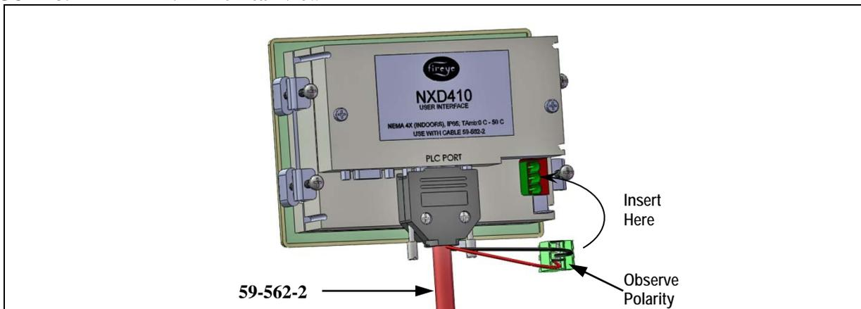
The bottom edge of the display must be mounted at least two inches from any cabinet door edge to allow sufficient clearance for the 59-562-2 cable.
