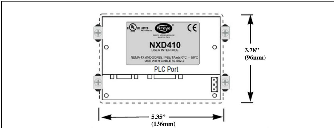
Use Fireeye cable, part number 59-562-2 to connect from the NXD410 to the PPC4000 control. The DA15-FM connector plugs into the PLC port located on the backside of the NXD410. The cable distance from the PPC4000 to the NXD410 is limited to 10 feet (3 meters) wire run.
