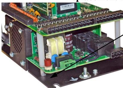
23-227, F1 Main input protection fuse, 5A, 250VAC, radial can
