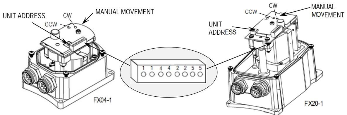
**WARNING** - DO NOT USE THE MANUAL MOVEMENT SWITCHES ON THE SERVO MOTORS DURING AUTOMATIC OPERATION OR THE FIRING CYCLE OF THE BURNER. USE OF THE MANUAL MOVEMENT SWITCHES OPERATES THE SERVOMOTORS INDEPENDENT OF THE PPC4000 CONTROL AND COULD RESULT IN AN OFF-RATIO CONDITION IF OPERATED DURING AUTOMATIC OPERATION OR THE FIRING CYCLE
