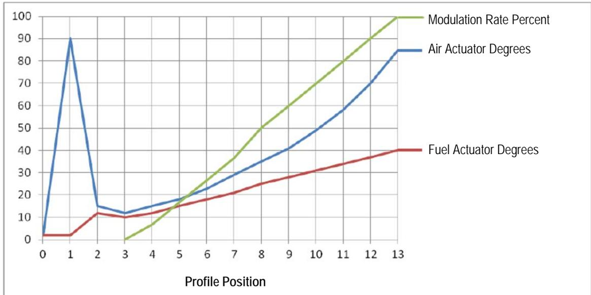
The reason for the difference between the two example curves is due to the AIR servo's upward curving slope but the FUEL servo's slope is straight. The modulation rate curve will resemble the curve of master servo.
