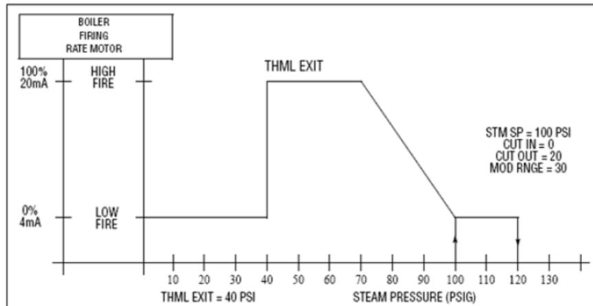
**SEGMENT METHOD:** This method of cold start thermal shock protection is generally used with Fire Tube Boilers. The setpoints associated with this method of thermal shock protection are:
