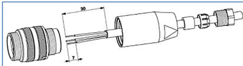
As shown above the cable strip length is specified at 30 mm (1.2 in) and each wire strip length is 7 mm (0.275 in).
