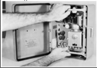
2. Wiring Changes: It is necessary to isolate the running interlock (air flow switch) from the low fire start switch. After isolating the circuits, reconnect the low fire start switch between B and 8 and running interlock between R and 3 on CB-1 terminal board. See Figure 1.
