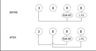
**3.** Note the typical diagrams figure for complete information. Install the Modernization Adapter and tighten the two retaining screws.
