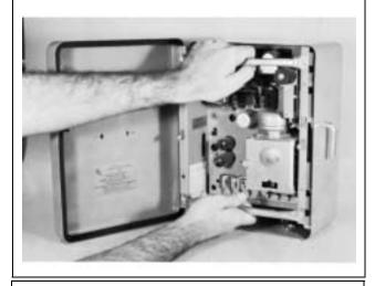
**5.** Install the Modernization adapter and tighten the two retaining screws.
