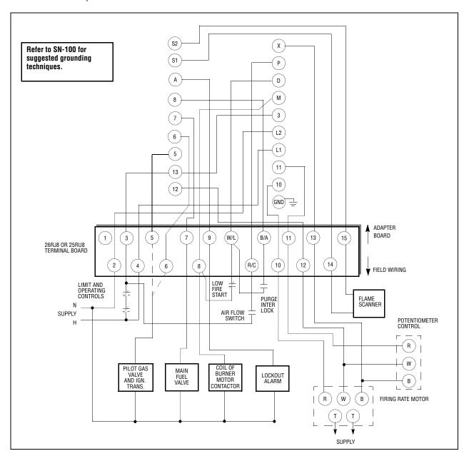
**Note:** For systems with ignition connected to terminal 1, disconnect and move to terminal 5. For early spark termination, replace EP160 with EP170, move ignition transformer to terminal 5 and pilot valve to terminal 6.
