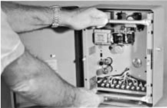
2. Fireeye 25SU5 controls may be wired and operated in a variety of methods. The circuit diagram on page 3 illustrates the interconnection between the 25SU5 and 70D40-41 control. It shows the recommended method of connecting the supply, limit switch, and momentary start switch, as well as the two SPDT relay circuits whose function is the same for both 25SU5 and 70D40-41 controls. All wiring must have 600 volt insulation.
