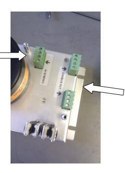
Connect CanBus out to addition servomotors.
