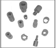
Fireye offers an extensive line of servomotor shaft couplings. Each coupling has flatted "D" holes on both the motor and driven shaft end. Available in a wide range of sizes these couplings, when used with the available shaft filing guide, assure a direct connection that will not rotate even if the setscrews loosen. For FGR damper applications, where thermal expansion of the damper shaft may cause thrust loading of the motor shaft, Fireye offers a unique expandable flexible coupling.
