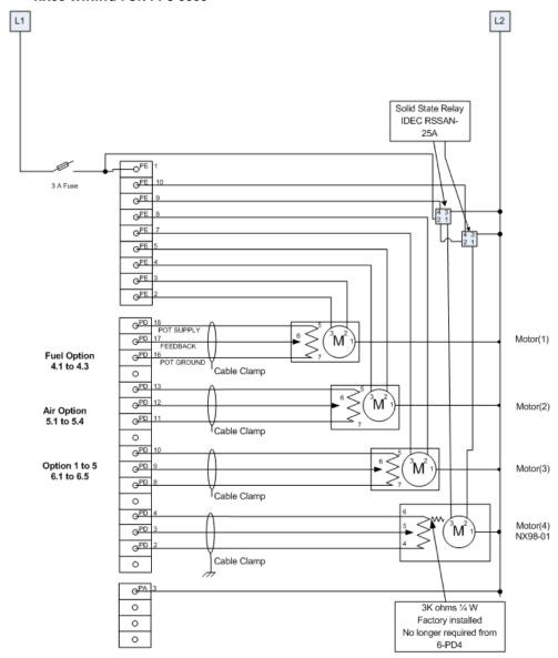
**Note:** Prior to the date code 0630, the 3K ohm resistor was supplied for external connection from the Potentiometer Supply to terminal 6 the NX98 motor. From the date code 0630, the resistor is supplied factory mounted between terminal 6 and the input to the feedback pot as shown above.
