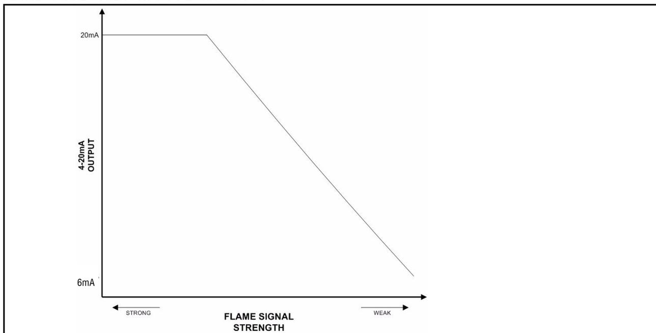
4-20mA measurements can be taken from the test jack connector located at the faceplate of the unit. Measurements can also be taken using the dedicated 4-20mA OUT & 4-20mA COM terminals located at the wiring base.
