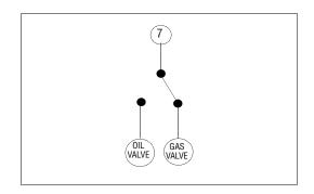
When changing fuels on combination oil and gas burners, **if** DIRECT SPARK IGNITION is used on oil and gas pilot is used on gas, wire as follows:
