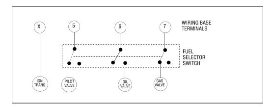
\*As shown, ignition spark on for 5 seconds. Option for 10 second spark, wire to terminal 5
