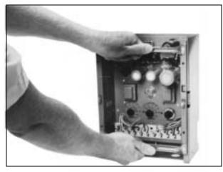
4. Insert modules in new Control chassis and install into Modernization Adapter. Tighten the chassis mounting screw.
