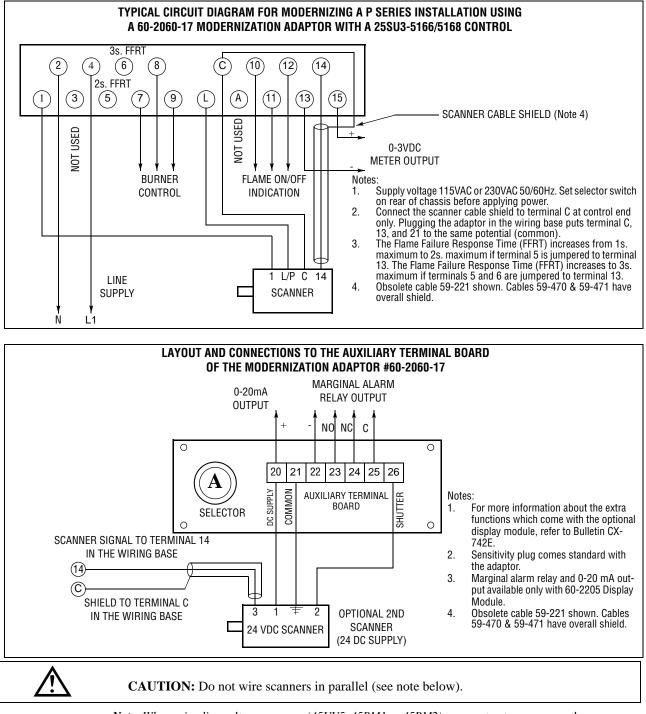
*Note:* When using line voltage scanners (45UV5, 45RM1 or 45RM2) you must not power more than on scanner from the same power (L) or shutter (1) terminal.
