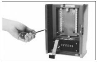
5. Remove the connector board cover at the bottom of the chassis.
