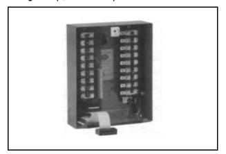
The wiring base is used to terminate all wires to the control. It should be mounted on a smooth, secure surface capable of supporting the base and control. The chassis and control assembly mounts into the wiring base and is secured using the single mounting screw. The ribbon cable included with the base should be plugged into the lower left corner of the chassis.
