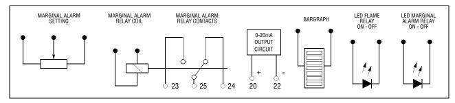
Remove the Blank Display Module from the chassis slot marked "Display Module" and replace with the Display Module, Fireye P/N 60-2205, shown above.
