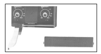
Install the chassis into the wiring base by aligning the two metal tabs on the wiring base with the cutouts in the chassis. Connect the chassis to the wiring base using the chassis mounting screw. Make sure that the mounting screw is fully tightened so that the chassis seats completely onto the wiring base.
