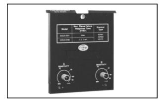
An indication of flame signal strength can be obtained using a remote meter (see Accessories on Page 14) or a 20,000 ohm per volt voltmeter on a 3 volt DC scale. Wire to the test jack terminals found on the face of the flame amplifier module or to terminals 15 and C/13.
