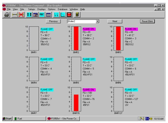
The Flame Quality is depicted as a value from 0 to 100. The scanner description, current file, Current Temperature and Comm Address are also shown.
