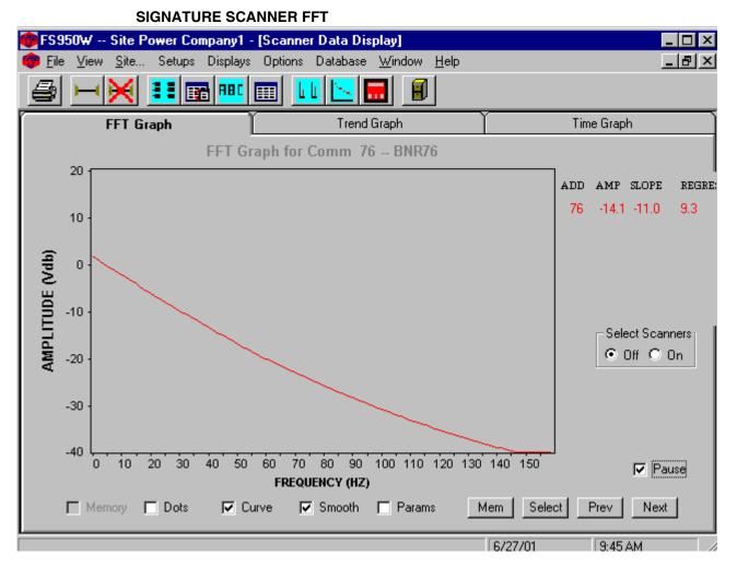
The Signature Scanner uses a 256 point Fast Fourrier Transform to analyze the data from the target flame. The FFT screen contains the graphic representation of those points.
